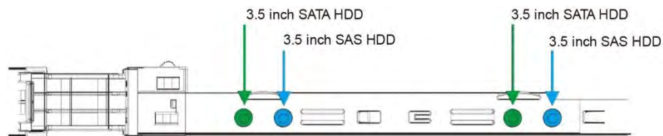
Installing a 3.5" SAS / NL-SAS / SATA Drive
