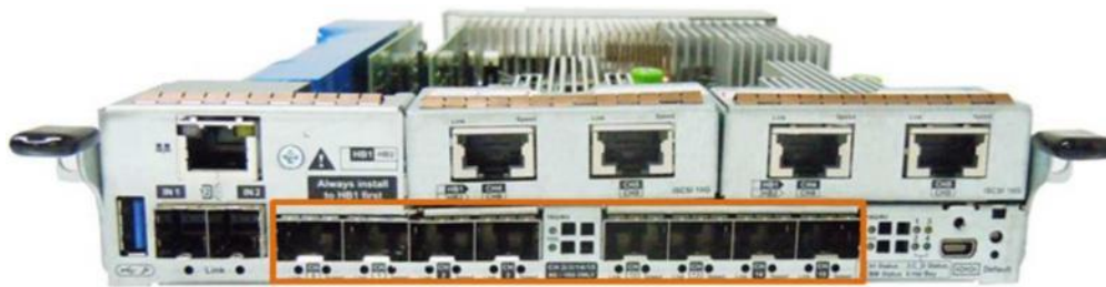
PS Gen2 4000 Dual Host Board and Embedded On-Board Converged Host Board Design
